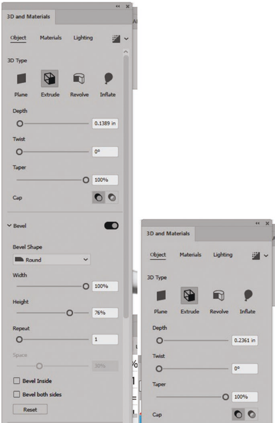
Figure 2-29. 3D and Materials Panel with Object Tab and a setting of Extrude for the circle and rounded rectangle
