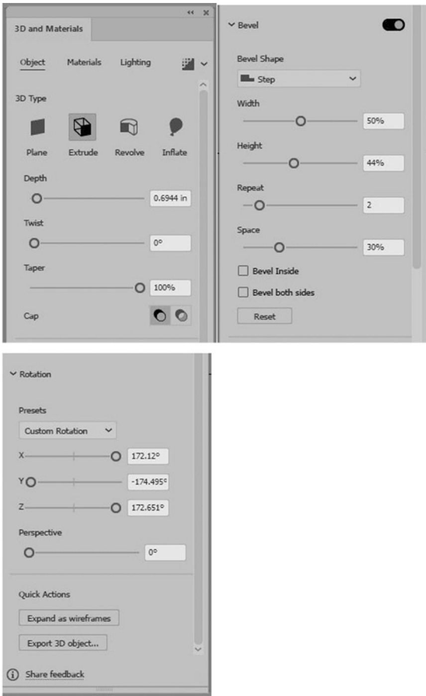
Figure 2-48. 3D and Materials panel with settings in the Lighting Object Tab for Extrude
